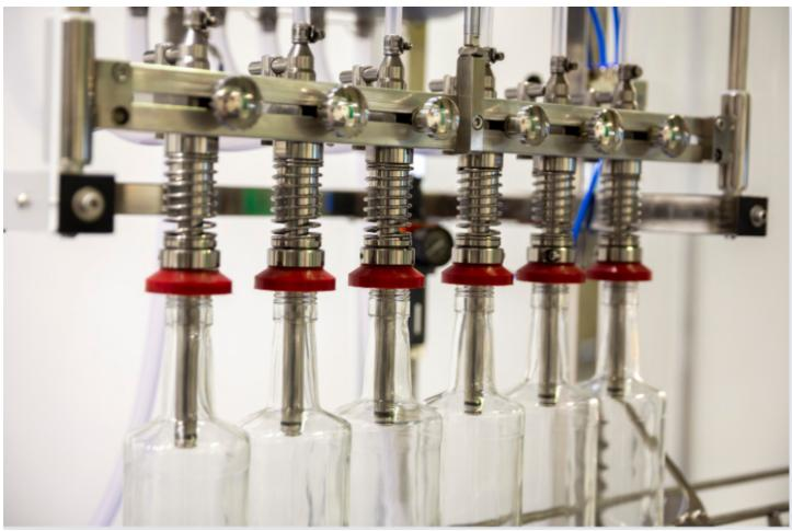
When comparing cosmetic products, pump filling machines are the most versatile fillers. They are perfect for a variety of products, including creams, lotions, gels, and water thin products. Pump filling machines are available in many types and sizes, including semi-automatic, two-head, and 12-head options. These machines also have touchscreen controls and Allen-Bradley PLCs.
