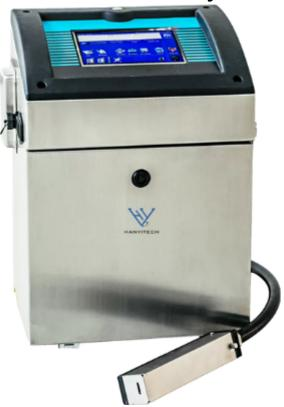
An industrial inkjet printer works on a principle known as a drop on demand. When an object is print printhead ejects a drop when the user requests it. The printhead has two different types of pressure one called thermal and one called piezo. Depending on the type of pressure pulse, the inkjet printer either a single color or a combination of colors.
