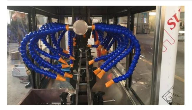
It replaces the traditional brush type dewatering device, does not need heating, and uses strong wind (air knife) to dry the bottle water. The bottle body is pollution-free, no need to replace the brush, no need to replace the electric heating tube, save the cost of use, and improve the performance. Advanced and more reliable.
