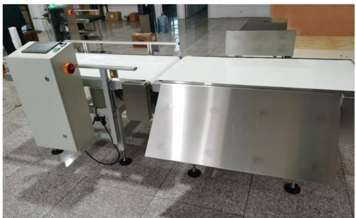
Large-scale re-inspection scale: According to the customer's product weight, product packaging size, and weighing efficiency, the specifications of the checkweigher can be customized. The size of the weighing platform covers 600mm\*400mm, 800mm\*500mm, 1000mm\*600mm, 1200mm\*600mm, 1400mm\*800mm and other large table weighing.
