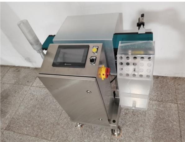
Capsule checkweighers are sensitive enough to detect weight changes of even a few milligrams, which means that packages of missing capsules will be detected and removed before they reach consumers. For pharmaceuticals, this is critical, as missing or overfilling will directly affect the effectiveness of the drug, leading to product recalls that damage the brand and reputation. It can also lead to catastrophic consequences for the end user.
