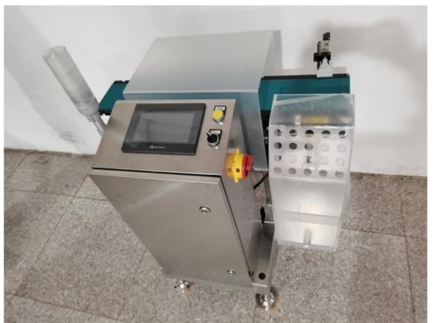
Capsule checkweighers are sensitive enough to detect weight changes of even a few milligrams, which means that packages of missing capsules will be detected and removed before they reach consumers. For pharmaceuticals, this is critical, as missing or overfilling will directly affect the effectiveness of the drug, leading to product recalls that damage the brand and reputation. It can also lead to catastrophic consequences for the end user.
