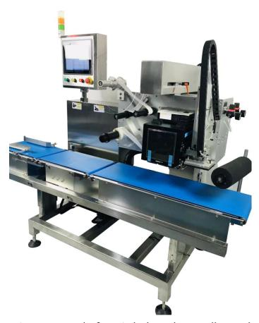
It is composed of static belt scale or roller scale (weighing range  $0\sim100$ kg, weighing accuracy  $\pm1/1000$  printing and labeling machine, fixed bar code scanner and industrial control computer.
