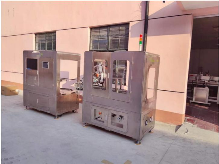
The working process of customized self-adhesive ampoule labeling machine is as follows: The robot picks up the material automatically ? Automatic printing ? Automatic labeling ? Visual detection rejection system ? Positioning of the product window ? Robot picks up the material automatically.
