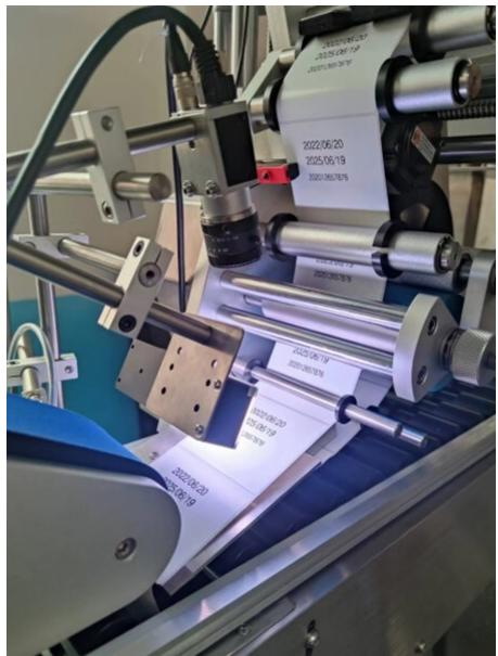
Automatic Horizontal Round Bottle Labeling Machine belongs to a series of round bottle labeling machines. Horizontal conveying and horizontal labeling method are used to improve stability and improve labeling efficiency.
