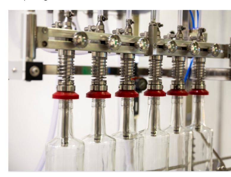
When comparing cosmetic products, pump filling machines are the most versatile fillers. They are pe a variety of products, including creams, lotions, gels, and water thin products. Pump filling machines available in many types and sizes, including semi-automatic, two-head, and 12-head options. These nalso have touchscreen controls and Allen-Bradley PLCs.
