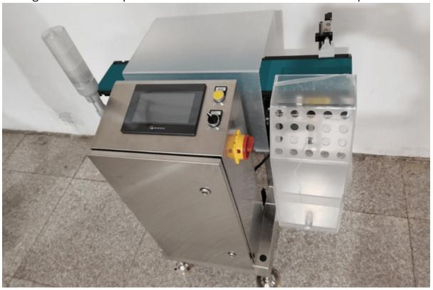
The High-accuracy Capsule Online Checkweigher can achieve accurate weighing and rejecting unqual products, so that pharmaceutical companies can calmly respond to the drug management law and d sampling management measures, and avoid being determined as inferior drugs due to different dose single capsule during quality sampling.
