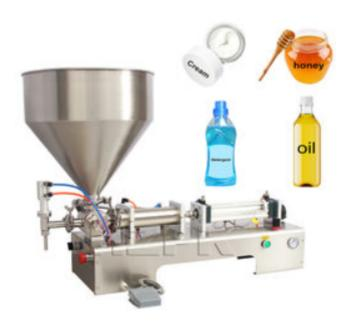
A tabletop piston filler will help you achieve greater efficiency in the filling process. They are designed to fill lotion bottles efficiently by shortening the fill time, and they feature a V-Groove Bottle Guide that helps you place the container under the fill head without spilling product. A tabletop piston filler is the perfect choice if you need a machine that will fill a large number of lotion bottles at once.
