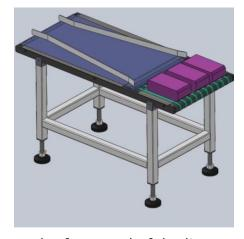
At the front end of the line combiner, the speed of the motors for the three lines can be adjusted (the knob adjusts the speed, and the speed of each line is different), and the three lines of products are combined into one line at the rear end of the line combiner.
