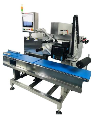
It is composed of static belt scale or roller scale (weighing range 0~100kg, weighing accuracy ±1/1000 printing and labeling machine, fixed bar code scanner and industrial control computer.
