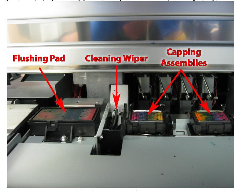
Regular maintenance is essential for all types of industrial inkjet printers. A daily maintenance schedulinclude cleaning the printer, replacing the ink, and replacing worn parts. To avoid clogging, it is recommended.
