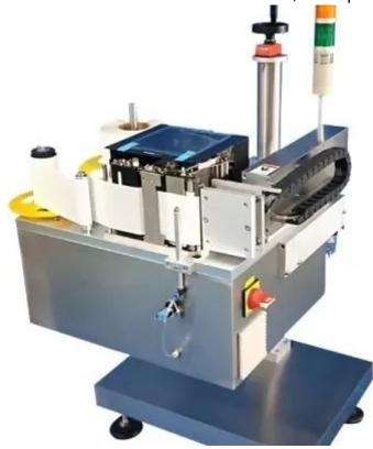
An automatic labeling machine has several parts. The chassis is a basic structure that supports other components. Most of them are made of stainless steel, and this helps them stay stable in a wide variconditions. The label trays are the second most important part of the labeling machine. Stainless steel a strong material and is resistant to a variety of elements. The final part of an automatic labeling syst printing heads.
