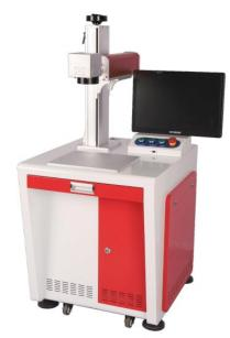
One of the first things to understand about a laser marking machine is how it works. The machine engraves an object onto a surface by focusing a high-power light on it. A controller is used to control the laser's movement across the surface of the material. The design file is used to program the machine's movements. During the process, the laser is aimed at the item, with the design file controlling the power of the beam.
