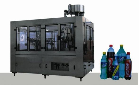
(1) The suspending bottle-necks cramping design makes the whole production line more stable during the working process and it also avoids malfunctions caused by the differences of thickness
