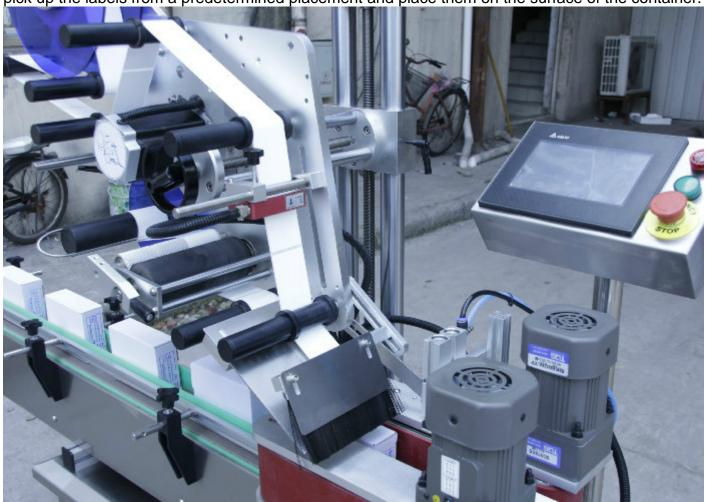
The labeling tape is dragged by a driving wheel, which pulls it out of the reel and presses the labels on the box. The machine uses a driving wheel and a reel to maintain the proper tension on the label tape. Because the labels are closely connected on the labeling tape, it must constantly start and stop to ensure proper application of labels. When a labeling machine is not properly working, it will fail to properly apply the label.
