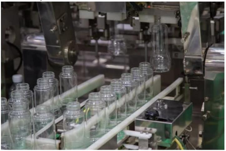
Pacific Packaging Machinery is the leading provider of rotary volumetric fillers for the personal care in These fillers feature four filling nozzle configurations for varying liquid flow rates, indefinite fill accurations time + pressure filling process. They are available with servo-powered positive displacement pumps to deliver speeds of up to 600 cpm. In addition, these fillers are designed for hygienic product environment feature stainless-steel components and NEMA 4X enclosures.
