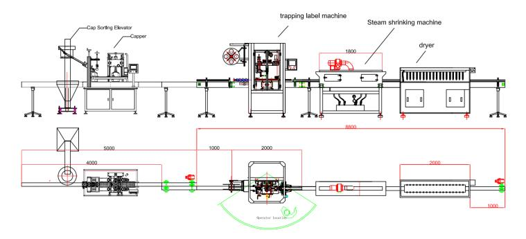
The label length is less than 80mm. The fastest production speed is 13000 bottles per hour, and the stable speed is 12000 bottles per hour
