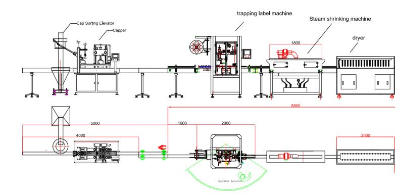
The label length is less than 80mm. The fastest production speed is 13000 bottles per hour, and the speed is 12000 bottles per hour
