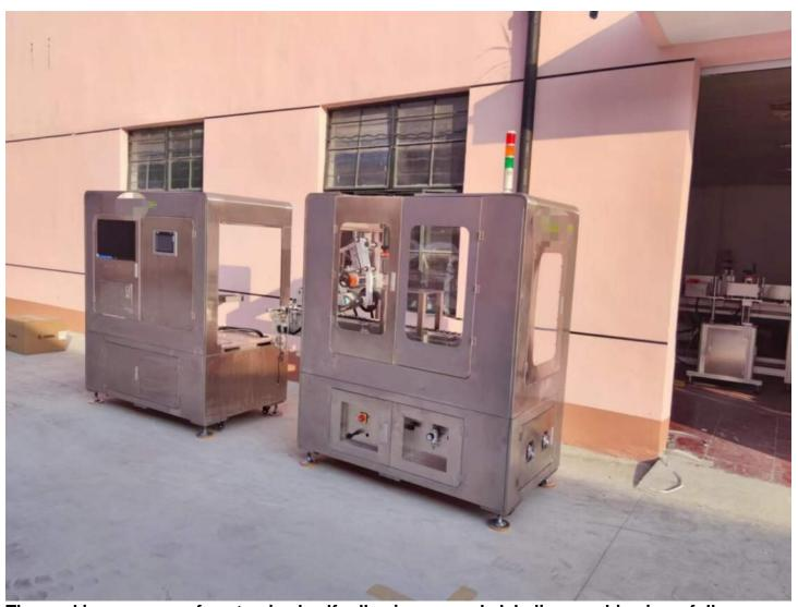
The working process of customized self-adhesive ampoule labeling machine is as follows: The robot picks up the material automatically? Automatic printing? Automatic labeling? Visual detection rejection system? Positioning of the product window? Robot picks up the material automatically.
