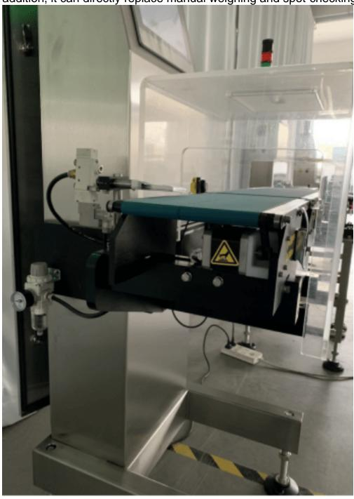
An automatic online weighing machine is suitable for the automatic weight detection of packaged products, as well as the quantitative detection of food, medicine, daily chemical products and other materials after packaging. Online check weigher can effectively re-inspect
