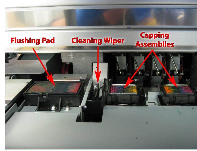
Regular maintenance is essential for all types of industrial inkjet printers. A daily maintenance schedu include cleaning the printer, replacing the ink, and replacing worn parts. To avoid clogging, it is recom
