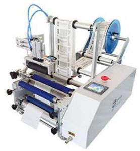
If you have been wondering how to use a semi-automatic labeling machine, read this article. This macapable of identifying and labeling bottles and other containers, including cylindrical and square bott also handle plastic, glass, metal, ceramic, and other materials. It can also label both the front and bac bottle. The maximum conicity is 1deg., and the sensors are critical for correct placement.
