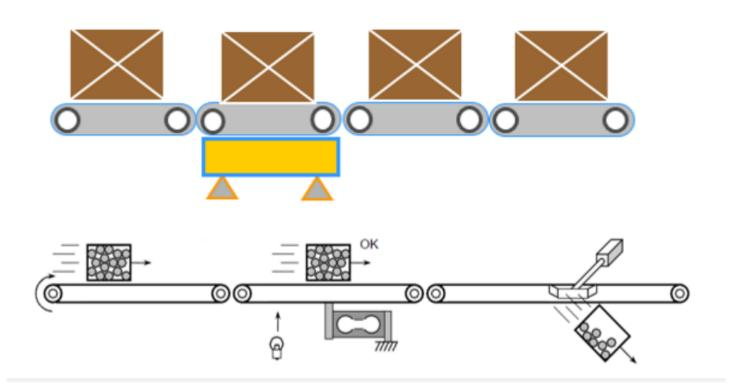
The fully automatic online weight detection equipment not only has high precision, but also greatly improves the efficiency. It can achieve 100% weight detection and save the original manual check weight. It can achieve 100% weight detection. In order to check the weight more quickly and accurately, we have also designed a double weighing platform, such as manual placement, which can be performed with both hands at the same time.
