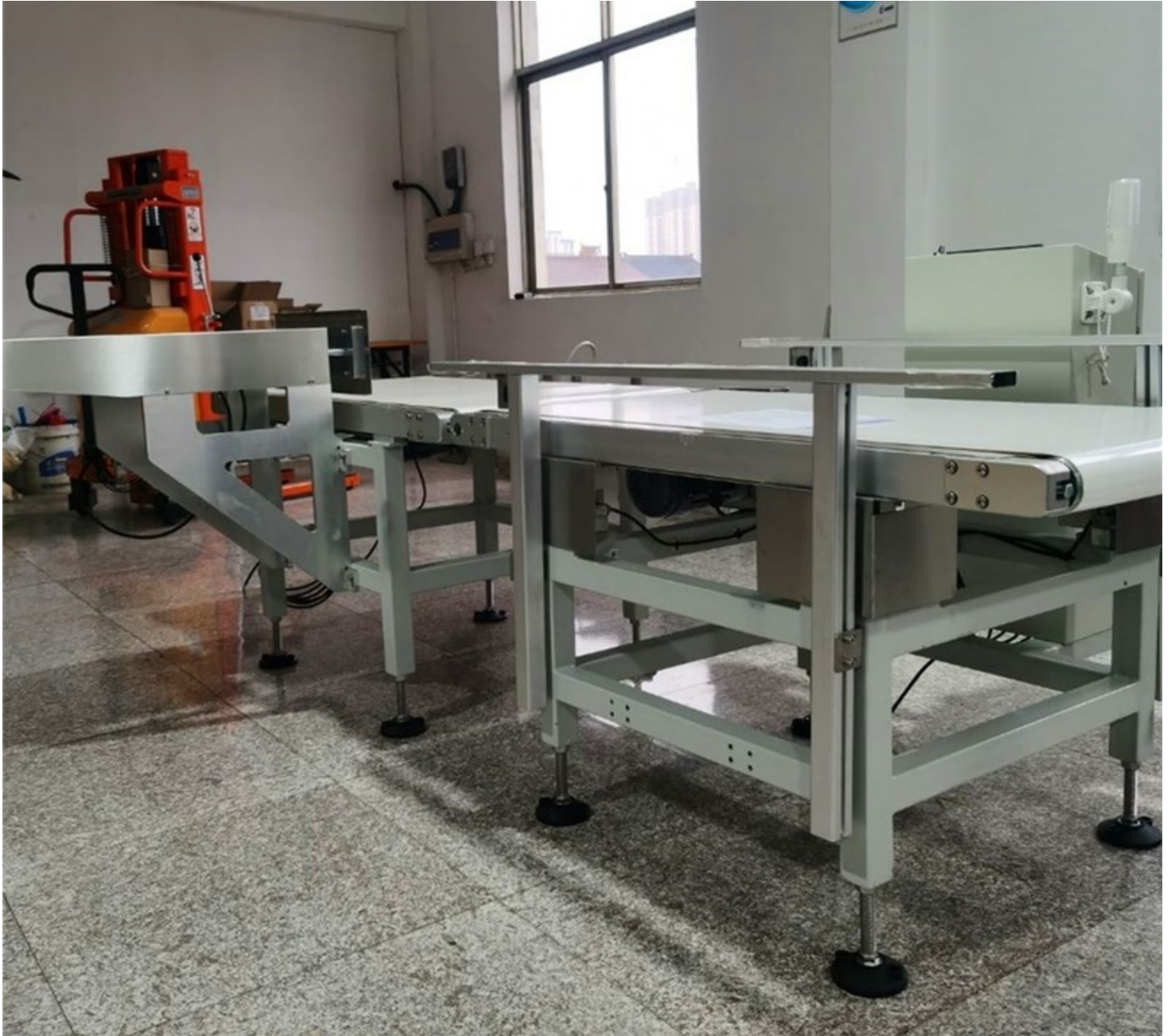
Large scale online weighing HYC50-12060 is widely used in pharmaceutical companies, food companies, daily necessities, chemical and other industries to meet the automatic and precise weighing of products in the automated production process.
