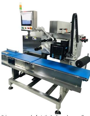
It is composed of static belt scale or roller scale (weighing range  $0\sim100$ kg, weighing accuracy  $\pm1/1000$ ), Hanyi printing and labeling machine, fixed bar code scanner and industrial control computer.
