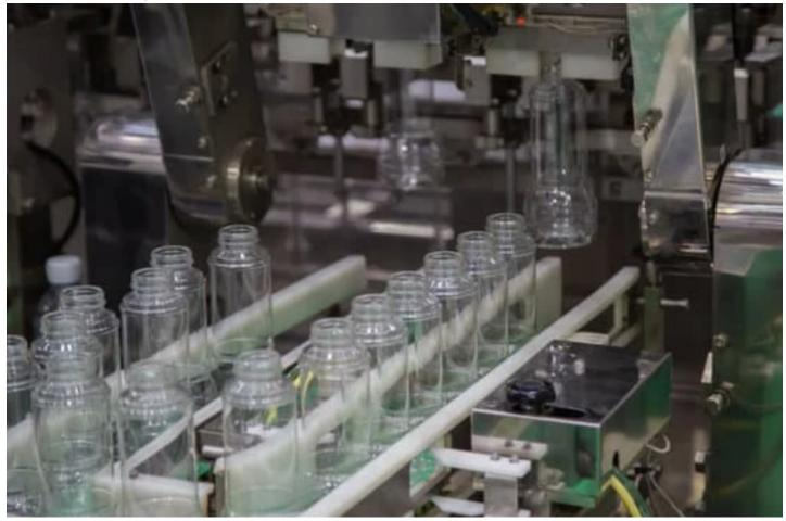
Pacific Packaging Machinery is the leading provider of rotary volumetric fillers for the personal care in These fillers feature four filling nozzle configurations for varying liquid flow rates, indefinite fill accura time + pressure filling process. They are available with servo-powered positive displacement pumps t deliver speeds of up to 600 cpm. In addition, these fillers are designed for hygienic product environm feature stainless-steel components and NEMA 4X enclosures.
