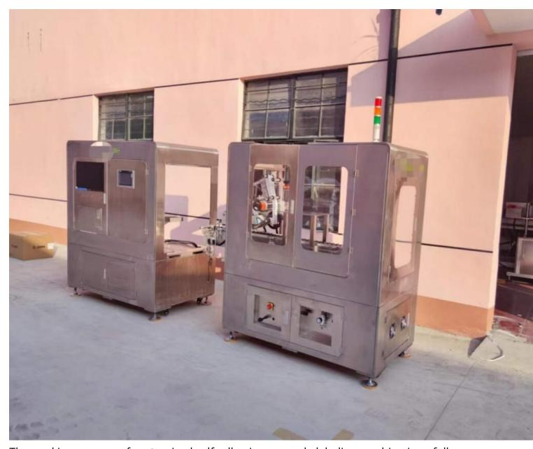
The working process of customized self-adhesive ampoule labeling machine is as follows:
