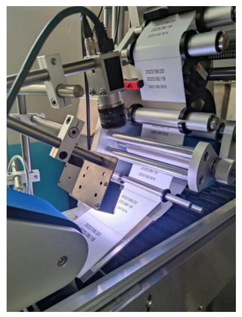
Automatic Horizontal Round Bottle Labeling Machine belongs to a series of round bottle labeling made Horizontal conveying and horizontal labeling method are used to improve stability and improve label efficiency.
