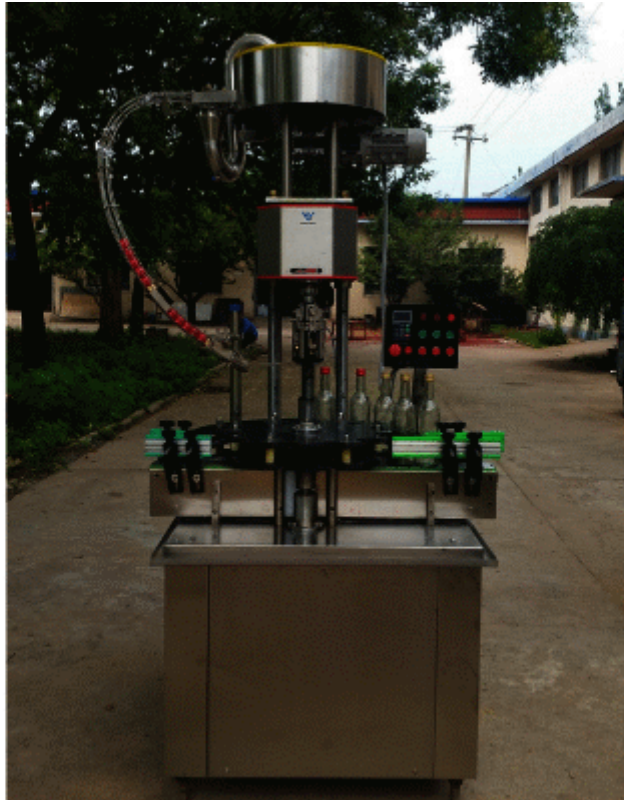
Single-head aluminum cap screwing machine
