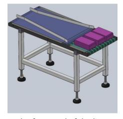
At the front end of the line combiner, the speed of the motors for the three lines can be adjusted (the knob adjusts the speed, and the speed of each line is different), and the three lines of products are combined into one line at the rear end of the line combiner.
