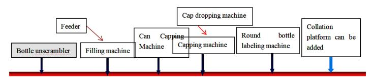
**Project Introduction:** According to customer requirements, this project will manually put the bottles to the production line. The double-head four-scale vibrating filling will automatically position and fill, and the automatic capping machine will automatically drop and cap.
