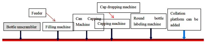
**Project Introduction:** According to customer requirements, this project will manually put the bottles to the production line. The double-head four-scale vibrating filling will automatically position and fill, and the automatic capping machine will automatically drop and cap.
