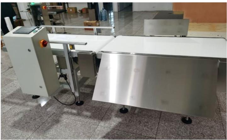
Large-scale re-inspection scale: According to the customer's product weight, product packaging size, and weighing efficiency, the specifications of the checkweigher can be customized. The size of the weighing platform covers 600mm\*400mm, 800mm\*500mm, 1000mm\*600mm,
