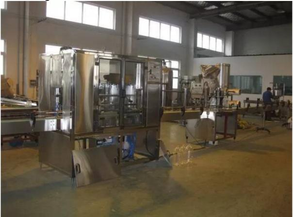
This filling line specially for 3-5gallons barreled drink water, with type QGF-100, QGF-240, QGF-300, QGF-450, QGF-600, QGF-900, QGF-1200.
