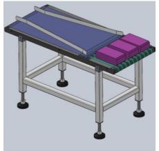
At the front end of the line combiner, the speed of the motors for the three lines can be adjusted (the knob adjusts the speed, and the speed of each line is different), and the three lines of products are control into one line at the rear end of the line combiner.
